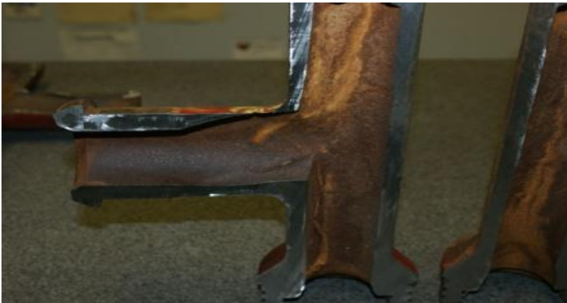
Washed Integral Elbow 5000psi. Wear Patterns are the same as Conventional Elbow. Washed to Atmosphere.
