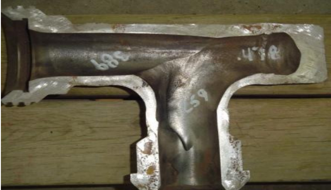
Another Conventional 5000psi fitting. Sand Cushion damage minimal. Again showing wear on both Bottom and Top side of Elbow
