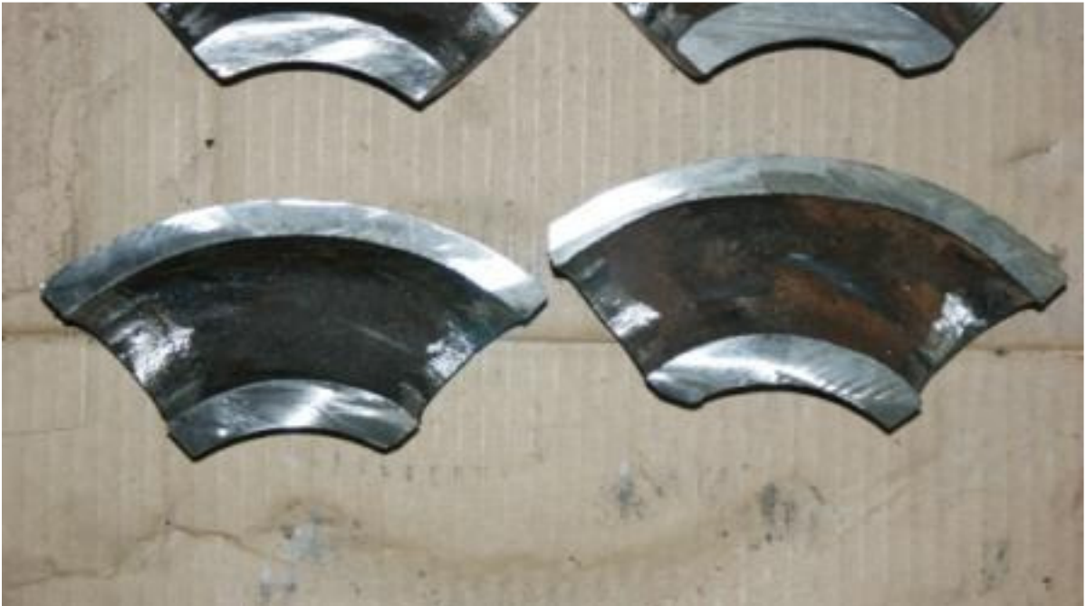
2" Schd#xxh has a wall thickness of .436 Cut 2" Elbow Outer wall measures .400
