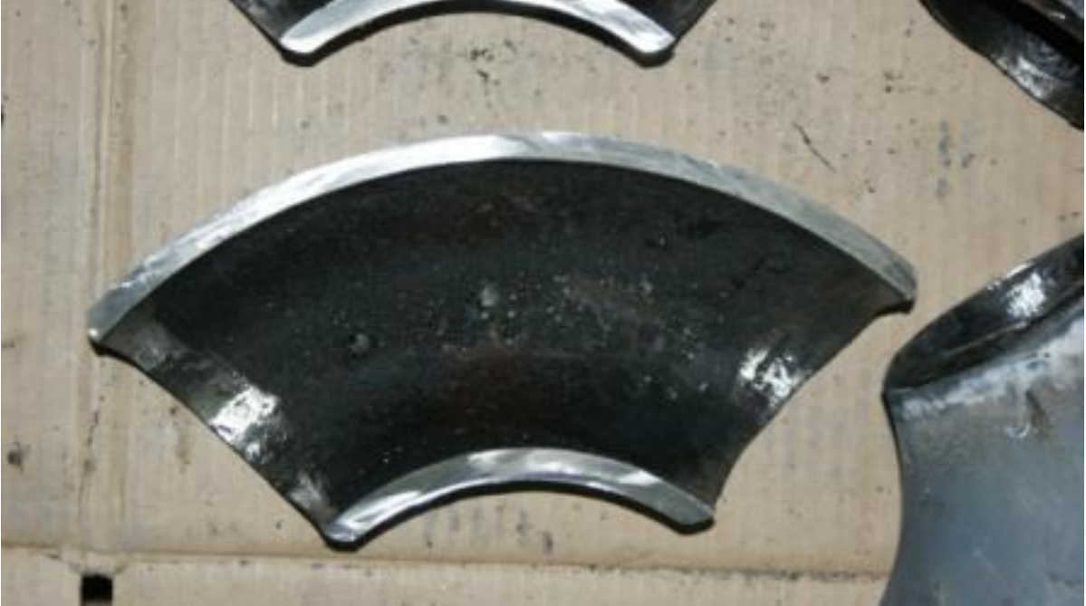
3"Schd#80 has a wall thickness of .300 Cut 3" Elbow Outer wall measures .280 Wall thickness.
